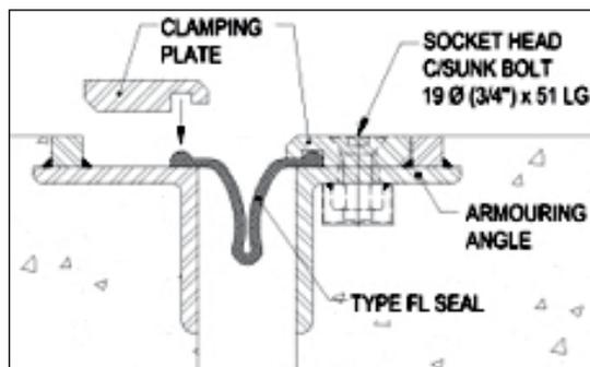
**FIGURE 1: Alignment of the seal bulge with the machined notch in the clamping plate**
