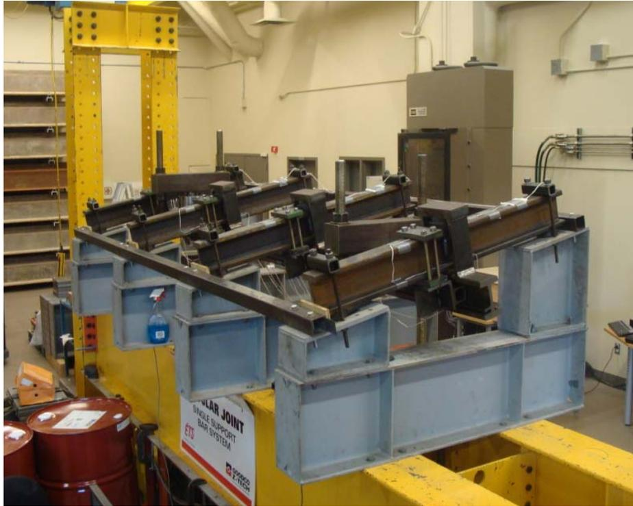
**Figure 3 – Instrumented Specimen Mounted on the Specially Designed Test Frame**
