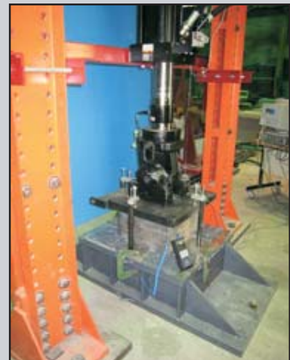
Dynamic test on vibration isolation bearings
