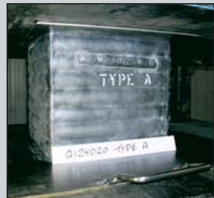
Static test on vibration isolation bearings
