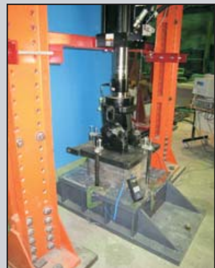
Dynamic test on vibration isolation bearings
