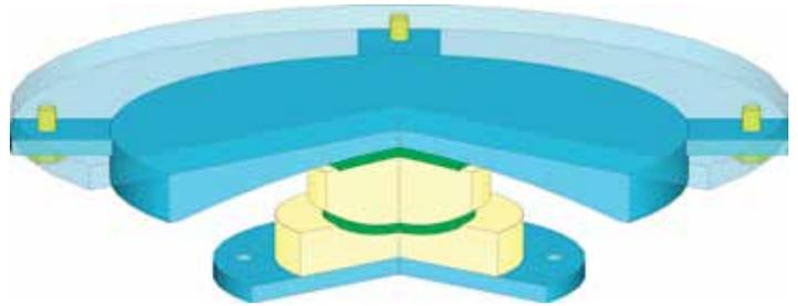
Figure 6: Friction pendulums rely on gravity to provide the restoring force. Since their lateral movement also creates a vertical movement, they must be installed throughout the structure. However, their period is a function of the radius of curvature radius only, which makes them a good alternative for light and heavy structures.
