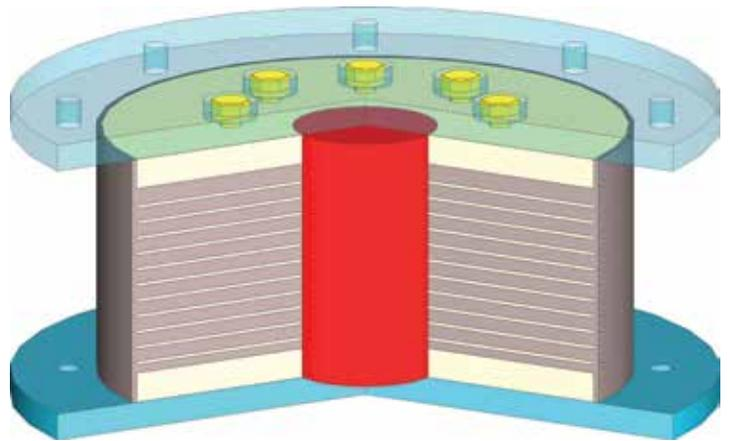
Figure 4: Lead-rubber bearings have a lead core that provides damping. Lead behaves as an elastic-plastic solid at room temperature and will regain its shape after deformation.
