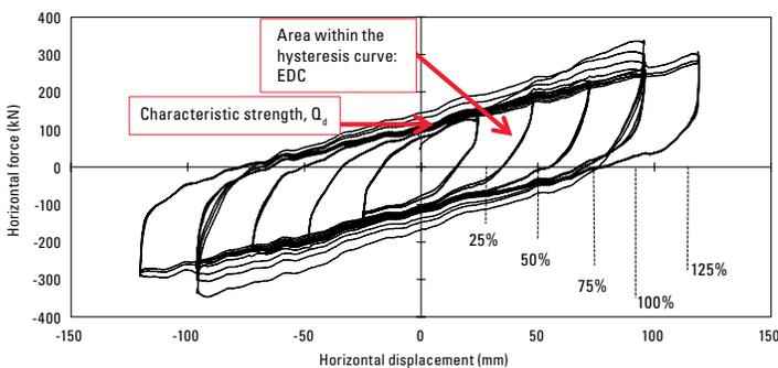
Figure 9: Force displacement curve during prototype tests of a lead-rubber bearing performed at room temperature, as specified in CAN/CSA-S6-06, section 4.10.11.2 c) ii).
