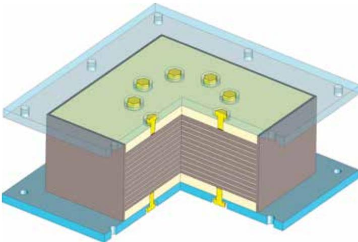
Figure 3: Elastomeric laminated bearing pads can be used to provide low damping for some projects. These bearing pads generally have a greater number of relatively thin internal layers compared to standard laminated bearing pads. They can be fabricated in a square or round shape. High-damping rubber bearings are constructed in the same manner.
