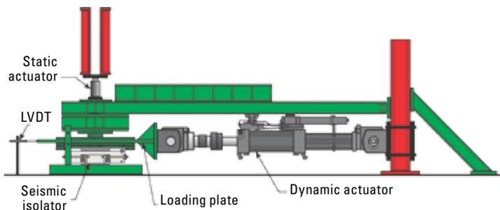
Figure 7: The test set-up at independent laboratory.
