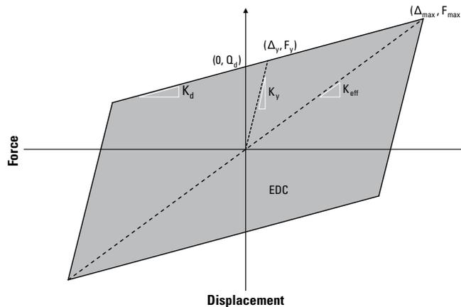
Figure 10: An idealized bi-linear hysteresis curve for a seismic isolator.
