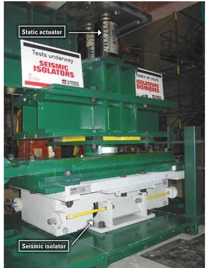
Figure 8: Z-Tech in a testing facility at independent laboratory.
