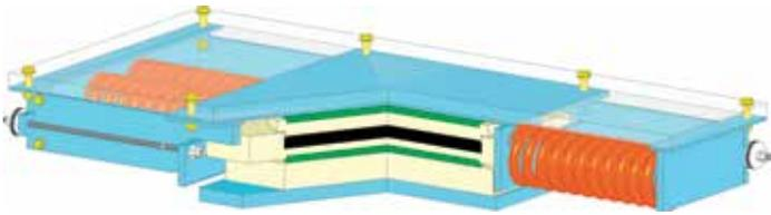
Figure 5: ZTS have high vertical load-carrying capacity and they can be designed with a wide range of damping values. The combination of the sliding interface and the spring elements provides a reliable energy dissipation system.
